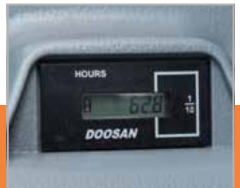
Hour meter (from ground level)
