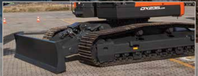
Highly durable dozer blade & undercarriage
